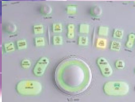
Operation panel customized for radiology examinations
